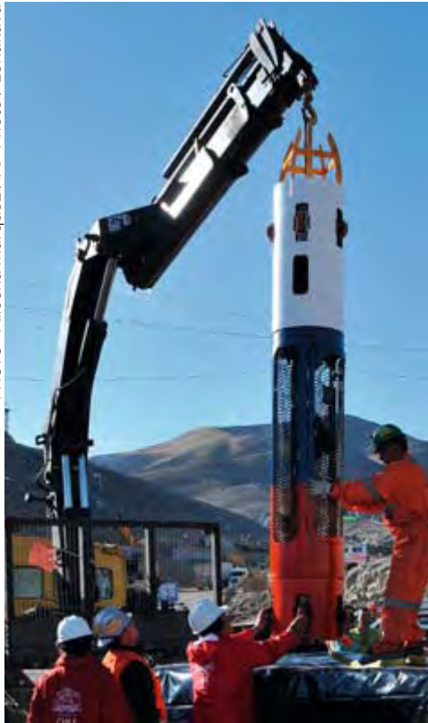
A Hiab XS 215 crane was used in test runs of the capsule supplied for the rescue operation in Chile that saved the lives of 33 miners trapped 7,000 metres underground. All men were brought to the surface on 13 October 2010 following 69 days in the mine.
